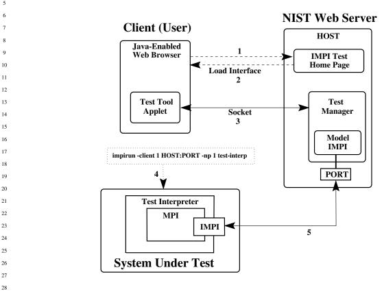
Figure 5.1: IMPI Test Architecture
