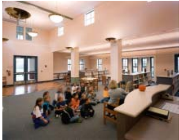
This library uses a combination of daylighting for ambient light and task lighting above desks and card files.
