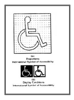
The placement of the access symbol is not specified by these guidelines. It is recommended that the symbol be placed at each accessible passenger door of an accessible vehicle. However, if the clear floor area for wheelchair or mobility aid users is provided at only one end of a car, then only those passenger doors at that location should be designated.
