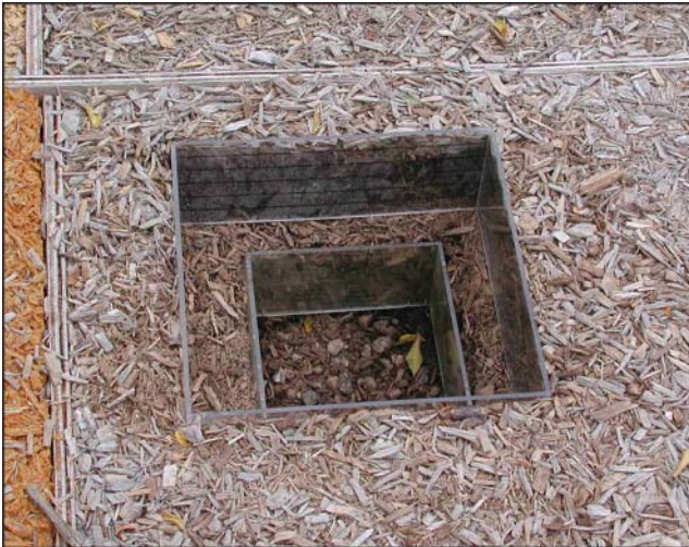
Figure 7—Archeological-type excavation for determining moisture profile of E2 surface. Note gravel at bottom of 0.3-m (12-in.) excavation.
