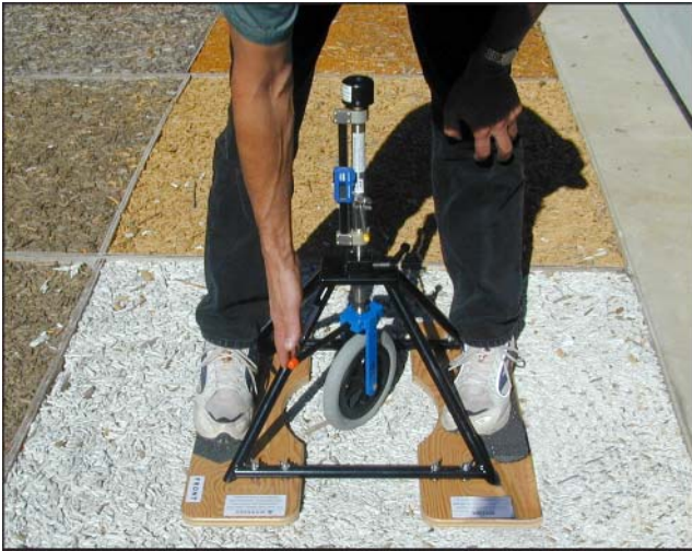
Figure 3—Rotational penetrometer in use on surface A2.
