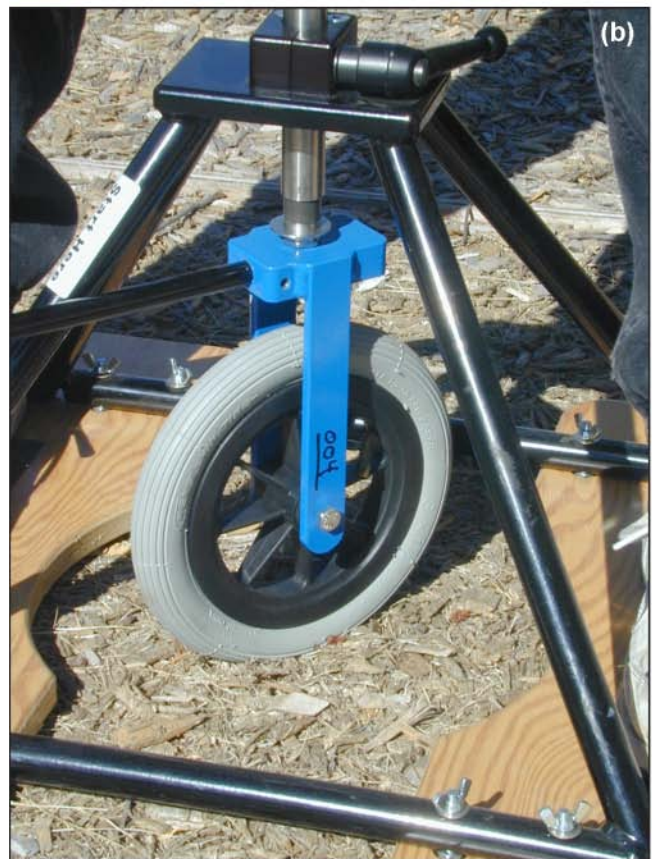
Figure 4—Accessibility test with rotational penetrometer. Stability readings taken after caster wheel was rotated 360°. (a) Poor stability of surface A2 indicated by amount of silicone-coated EWF displaced by rotated caster wheel; (b) good stability of surface G.
