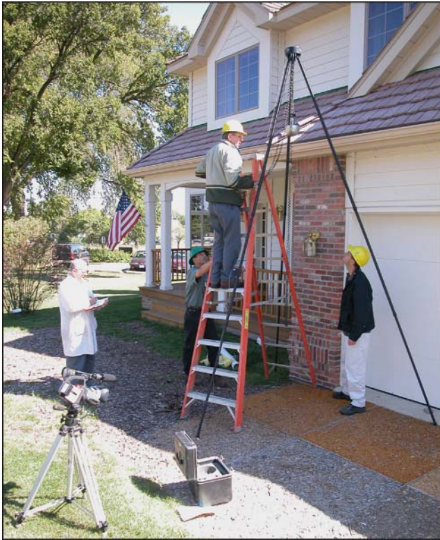
Figure 5—Impact attenuation test. A 4.5-kg (10-lb) hemispherical impact head was installed 3 m (10 ft) over surface D. Ted Illjes (on ladder) holds instrumentation package connected to impactor by coiled wire. Doug Zeager awaits arrival of impactor, which will be caught on first rebound from surface.
