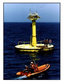
Source: USDOC, NOAA, NBDC 2008 Figure 3-8 A 10-Meter Discus-Shaped Hull Buoy
