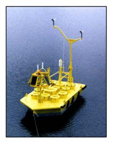
Source: USDOC, NOAA, NBDC 2008 Figure 3-9 A 6-Meter Boat-Shaped Hull Buoy (also known as a NOMAD)
