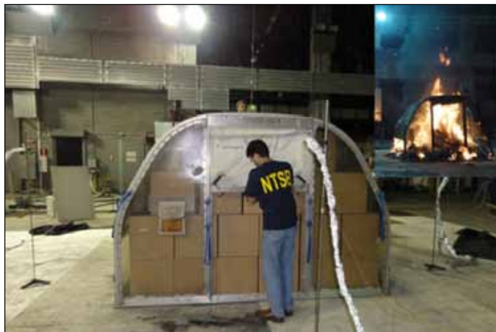
Figure 27. An NTSB fire and explosion investigator prepares a test at the fire laboratory of the Bureau of Alcohol, Tobacco, Firearms and Explosives to evaluate the fire detection systems of aircraft cargo bays. The inset photo shows the fire test underway.
