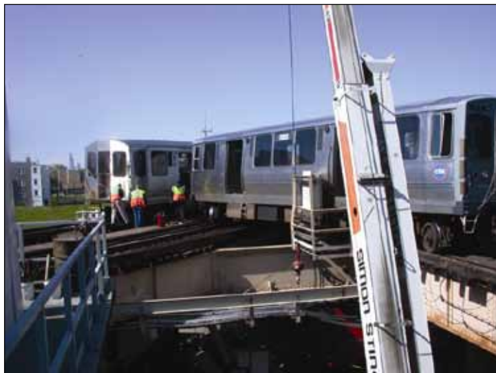
Figure 18. Derailed lead cars of Chicago Transit Authority.
