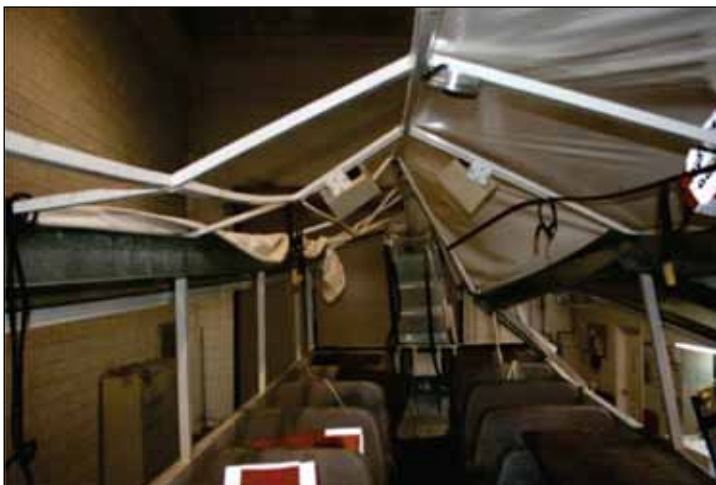
Figure 13. View of DUKW 34's damaged canopy, looking aft.
