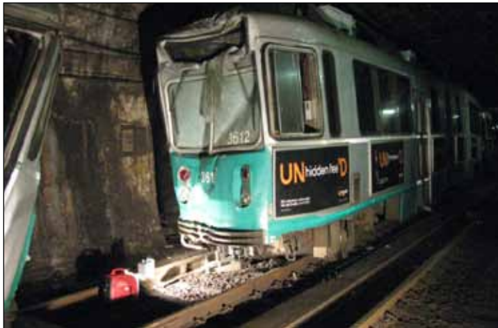
Figure 22. Damage to front (cab) train near Boston, Massachusetts.
