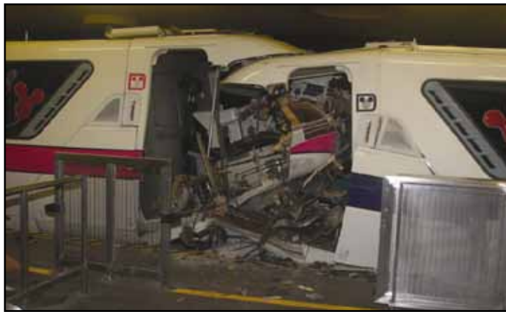
Figure 23. The accident monorails after the collision. The rear operating cab of the Pink monorail (unoccupied at the time of the accident) is on the left, and the front operating cab of the Purple monorail is on the right.
