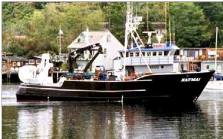
Figure 16. Fishing vessel Katmai motoring through Ballard locks in Seattle (undated Seattle Times photo). White cylindrical structure (net reel) at stern was later removed when vessel was refitted for cod fishing. Katmai was the only vessel owned and operated by Katmai Fisheries, Inc.
