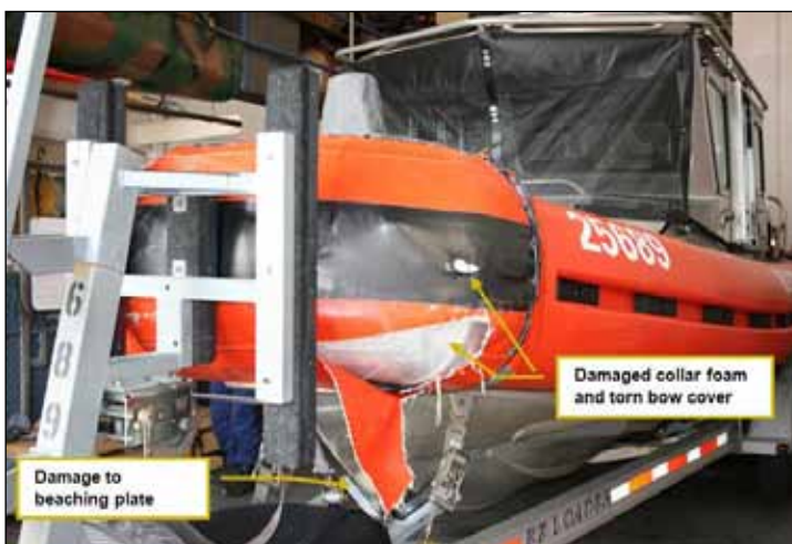
Figure 14. Damage to the CG 25689 's bow collar foam, bow cover, and beaching plate.
