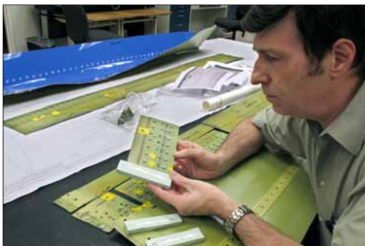
Figure 29: An NTSB metallurgist examines pieces of ruptured fuselage skin from a Boeing 737.
