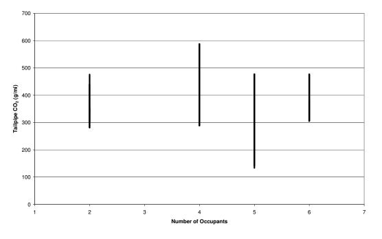
MY 2007 Cars: Range of Tailpipe CO<sub>2</sub> Emissions by Occupant Capacity
