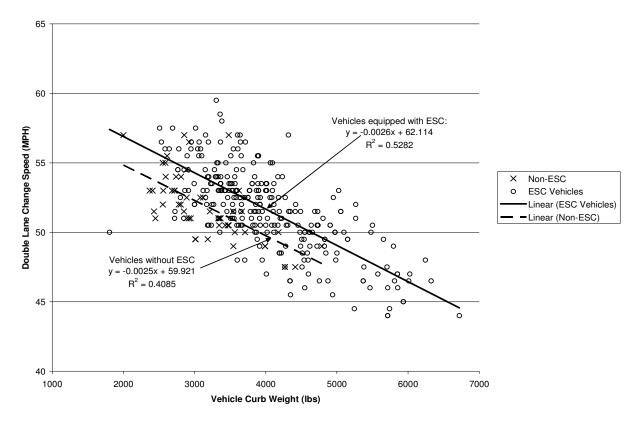
Figure 7-29 Double Lane Change Speed vs. Vehicle Curb Weight
