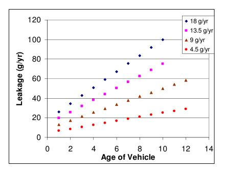
Figure 2-2 A/C Refrigerant Leakage Rate for Different Technologies as Vehicles Age
