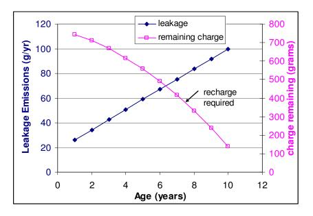
Figure 2-1 Deterioration Rate of Refrigerant Leakage
