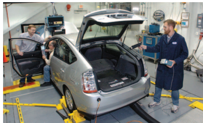
PHEV chassis dynamometer testing at Argonne National Laboratory’s Advanced Powertrain Research Facility.
