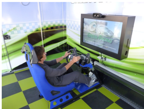
Figure 5. Lyn St. James, former Indy car driver, competing in the Green Racing simulator. The Green Racing simulator developed by Argonne incorporates a program that calculates the amount of regenerative braking energy captured and fuel used during two laps of simulated racing. This simulator was set up at five ALMS races in 2011. It served as a notable means of disseminating the DOE Green Racing's key message that the use of renewable fuels and hybrids can displace a substantial amount of imported petroleum.
