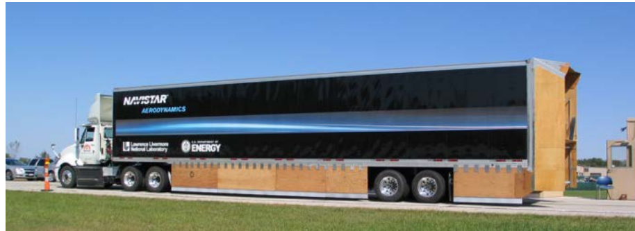
Figure 1. Track test vehicle equipped with a gap fairing, trailer skirts, and a trailer boattail.
