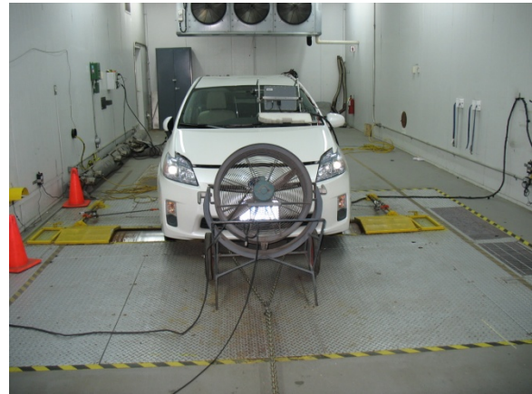
Figure 1. ANL-instrumented Prius in Environment Canada's thermal test cell
