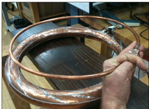
Figure 8. View of the wireless charging system showing the resonant antenna components. The top coil is the receiver that would be mounted to the vehicle, while the lower coil is the transmitter embedded in the floor or road bed.
