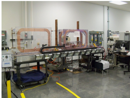
Transmit coils in background: ribbon coil (left) and copper tube coil (right) WPT Laboratory Apparatus with 3.3kW lamp load in foreground
