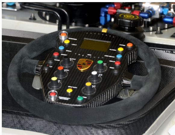
Figure 7. The steering wheel from the Porsche 911 GT3 R Hybrid. Note the extra dials to fine-tune the maps for hybrid components such as energy recovery, electric propulsion, and traction control close to the Porsche crest.
