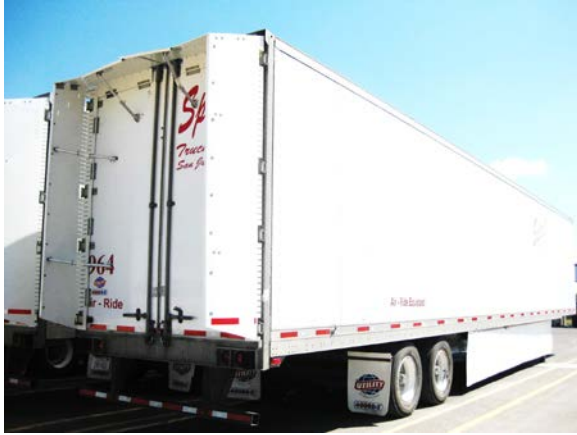
Figure 1. Freight Wing's advanced aerodynamic system to reduce the drag of the trailer, which is expected to yield fuel savings over 7% compared with the baseline.
