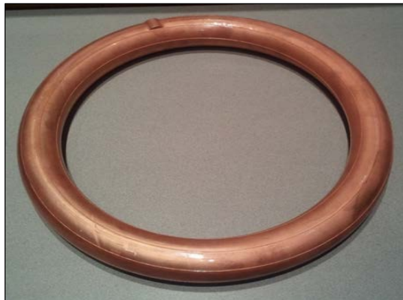
Figure 7. Hollow core primary resonance coil antenna design for low-cost manufacture.
