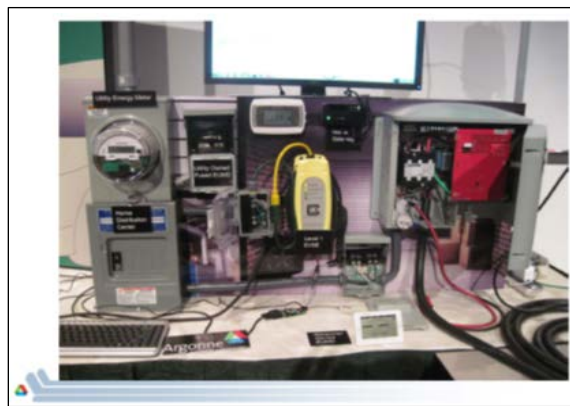
Figure 3. Table-top display to demonstrate Smart Grid interoperability, developed by Argonne.
