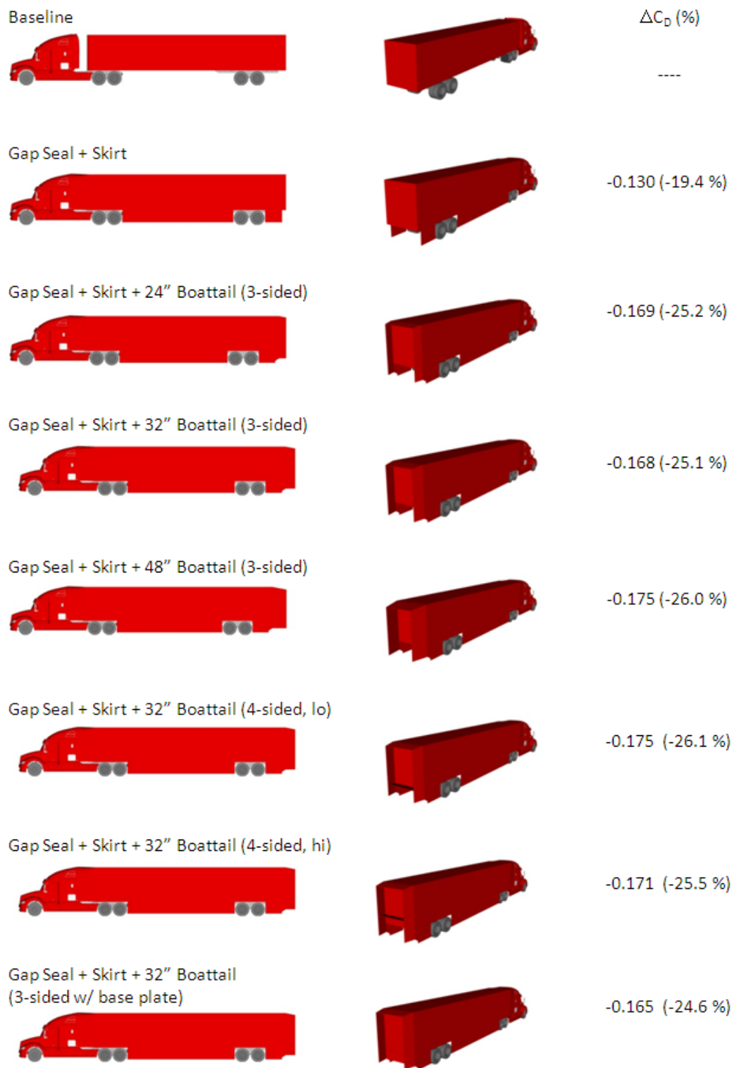
Figure 3. Heavy vehicle configurations modeled using computational fluid dynamics simulations. The trailer skirt and boattail devices are representative of those evaluated in a track test.
