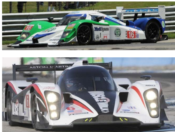
Figure 1. Five of nine LMP Green Challenge winners used advanced fuels. Photo of the Season and Green Racing Champion Dyson Mazda turbocharged 2-liter fuel with isobutanol (top) and the Pickett Aston Martin naturally aspirated V12 fueled with E85 (bottom).
