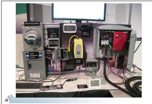
Figure 3. Smart grid interoperability demonstration bench.
