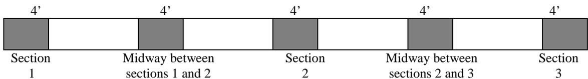
(c) **Loading Precautions for Vehicle Scales, Axle-Load Scales, and Combination Vehicle/Livestock Scales.** – When loading the scale for testing, one side of the test pattern shall be loaded to no more than half of the concentrated load capacity or test load before loading the other side. The area covered by the test load may be less than 1.2 m (4 ft) x 3.0 m (10 ft) or the width of the scale platform, whichever is less; for test patterns less than 1.2 m
