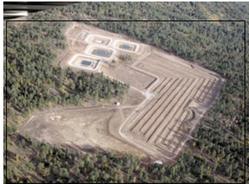
Figure 15: Overview of constructed fermentation pits/outer ponds to the upper left, constructed wetland channels to the right, and discharge out-fall to the lower left.
