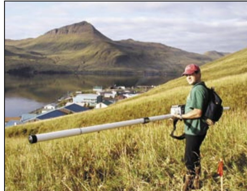
Figure 38: Engineer Kelly Leseman conducting an electro-magnetic survey at a potential water tank site.
