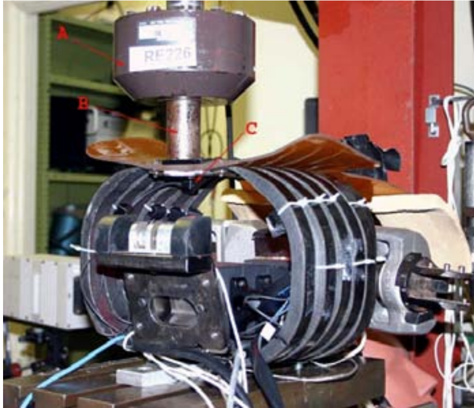
Figure 46: Test configuration for rib-mounted loading. A: indenter load cell, B: indenter, C: LED at right front end stiffener plate at the fourth rib.
