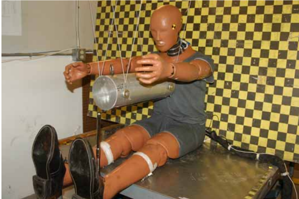
Figure 64: Hybrid III dummy set-up for neutral position pendulum testing according to CFR § 572.34
