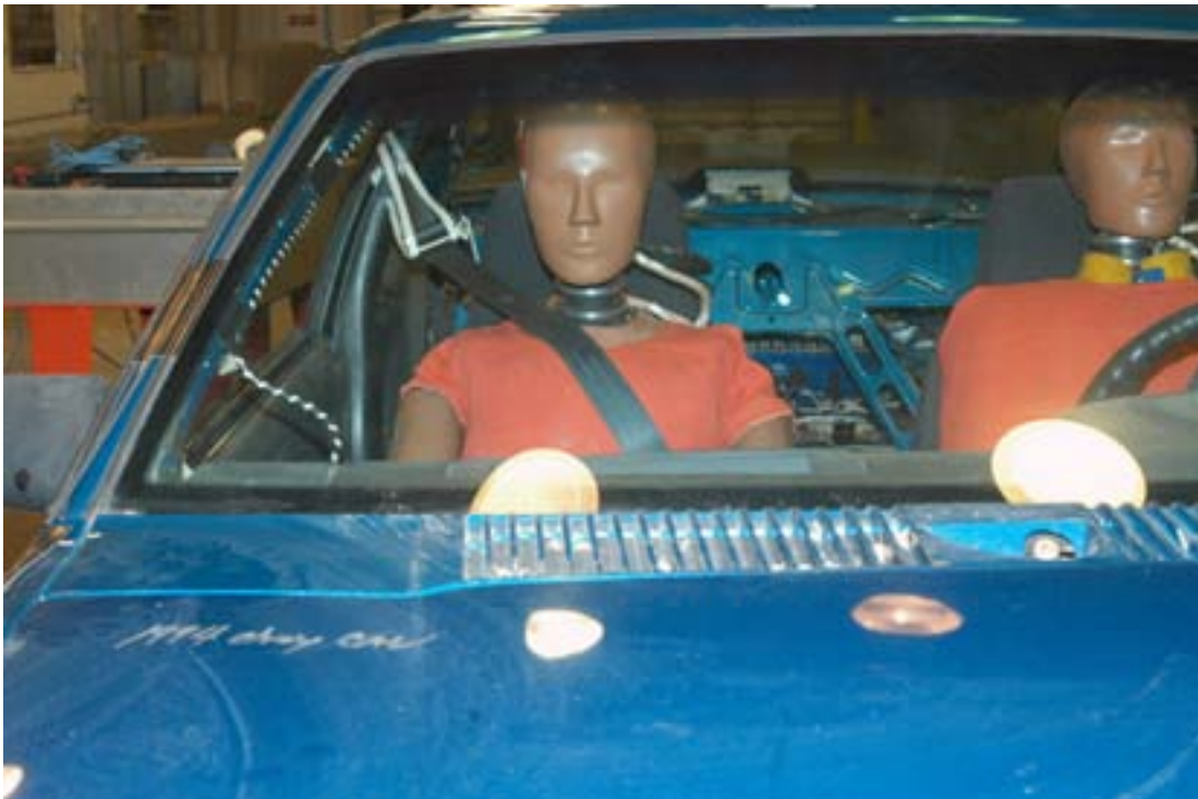
Figure 77: Photograph of pre-test position of Hybrid III/RibEye dummy in offset frontal crash test.
