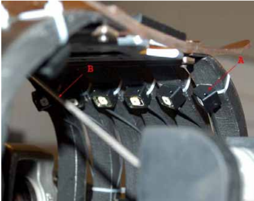
Figure 12: Photograph showing the LED fixation method at the 9 cm position. An LED is attached to the left fourth rib (A). The slide arm of the internal chest potentiometer is shown (B).
