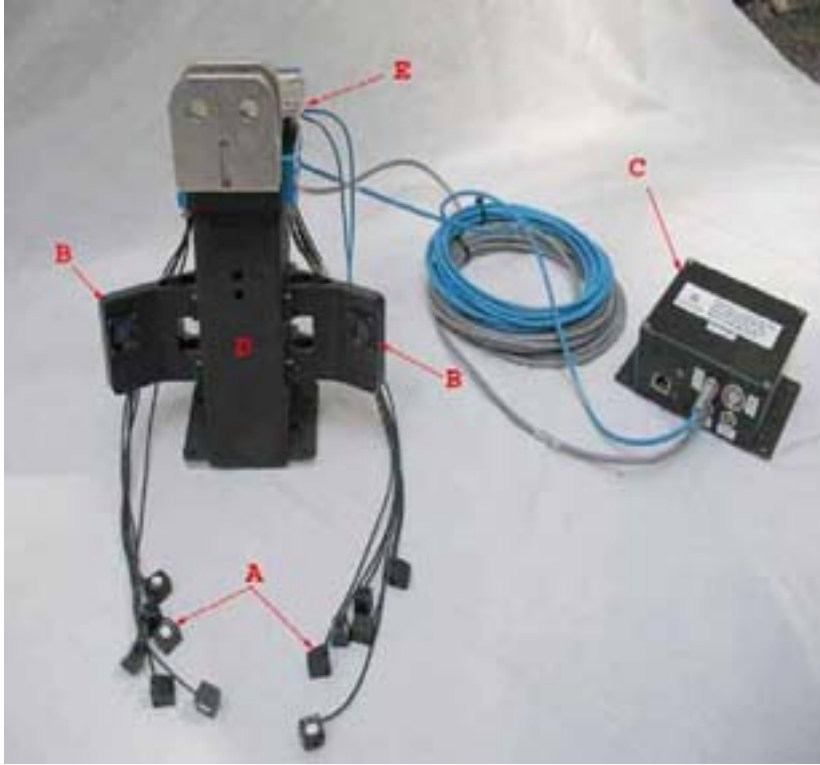
Figure 1: RibEye system showing the LEDs (A), two sensor heads located on either side of the dummy thoracic spine (B), interface box (C and E), dummy thoracic spine box (D), and LED connector block (F).
