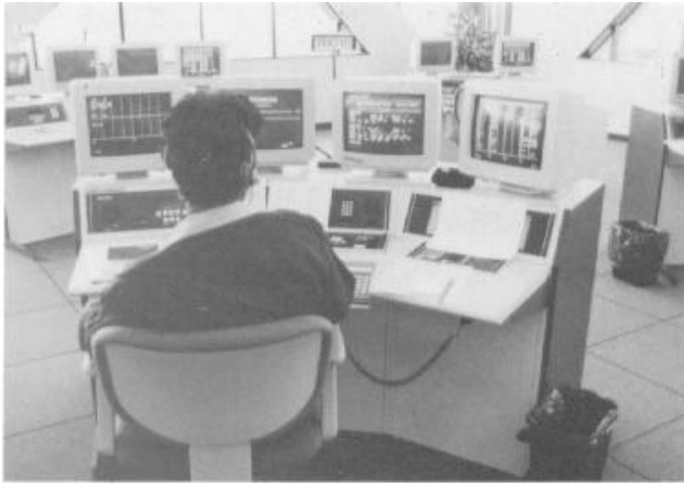
Exhibit 3-5. Los Angeles County CAD System display monitors at a Tactical Radio Operator Console.
