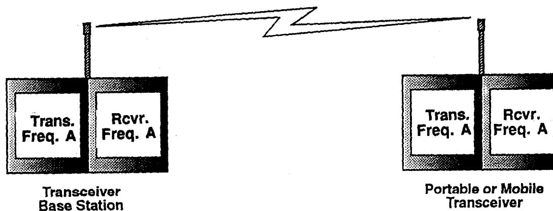
Exhibit 3-1. Transmitter Sections & Receiver Sections of All Transceivers on Same Frequency, Freq. A.
