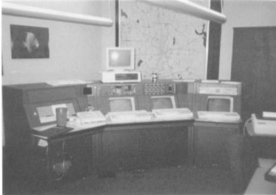
Exhibit 2-5. Dallas Fire Department Communications Center Training Console. The console allows realistic training without having to tie up an operational console.
