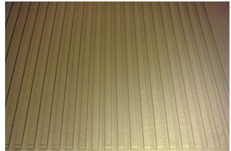
Bipolar plate channels, nitrided plate
