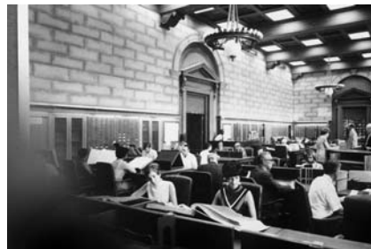
FIGURES 14-16 Traditional supplemental lighting such as desk lamps preserve the architectural dominance of historic chandeliers and place light where it is needed to perform work. Top (before restoration): Surface mounted fluorescent lighting compromises the reading room’s coffered ceiling and competes with the chandeliers. Middle and Bottom (after restoration): Reader-controlled desk lamps eliminate the need for high ambient light levels, enabling the ceiling to be restored to its original appearance.
