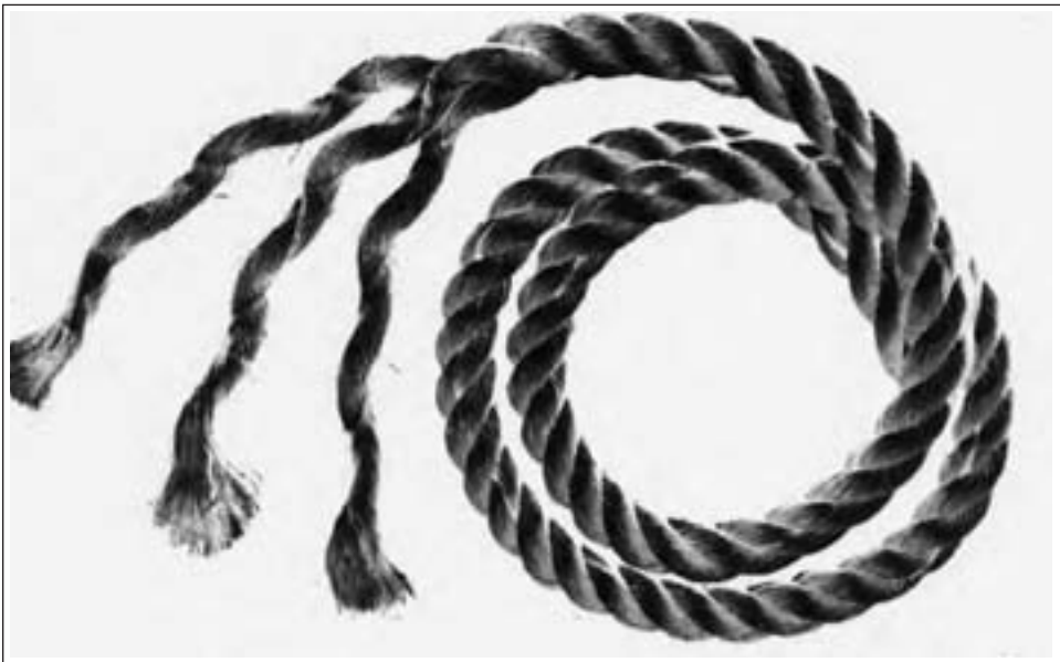
Figure 3.1: Hemp rope illustrating cord construction - filament/yarn/cord (rope)
