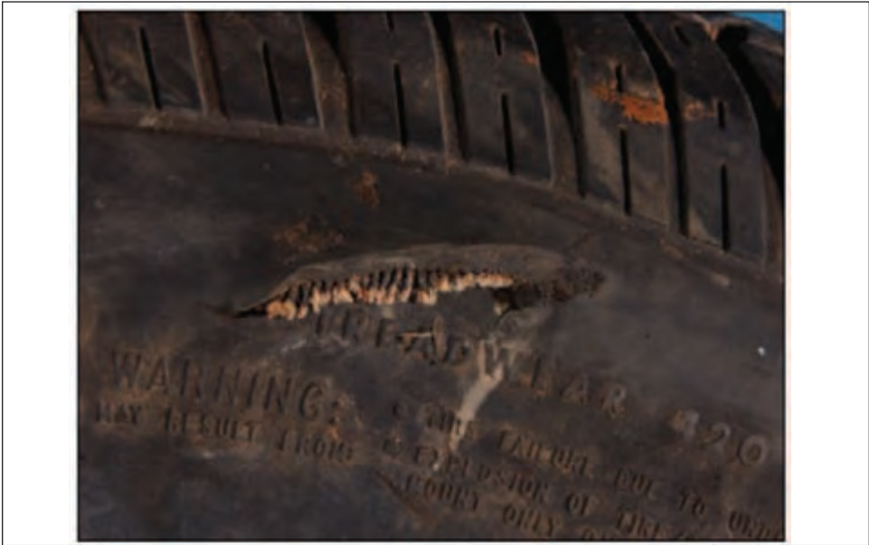
Figure 15.17: Upper sidewall break through to cavity
