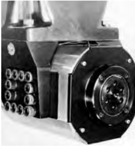
Figure 8.16: Unitary measuring head from a flat-trac II
