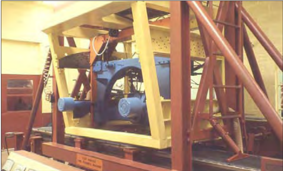
Figure 7.15: A modern, moving carriage, stationary bed, flat-surface machine manufactured by MTS Systems, Inc Bridgestone/Firestone Co.
