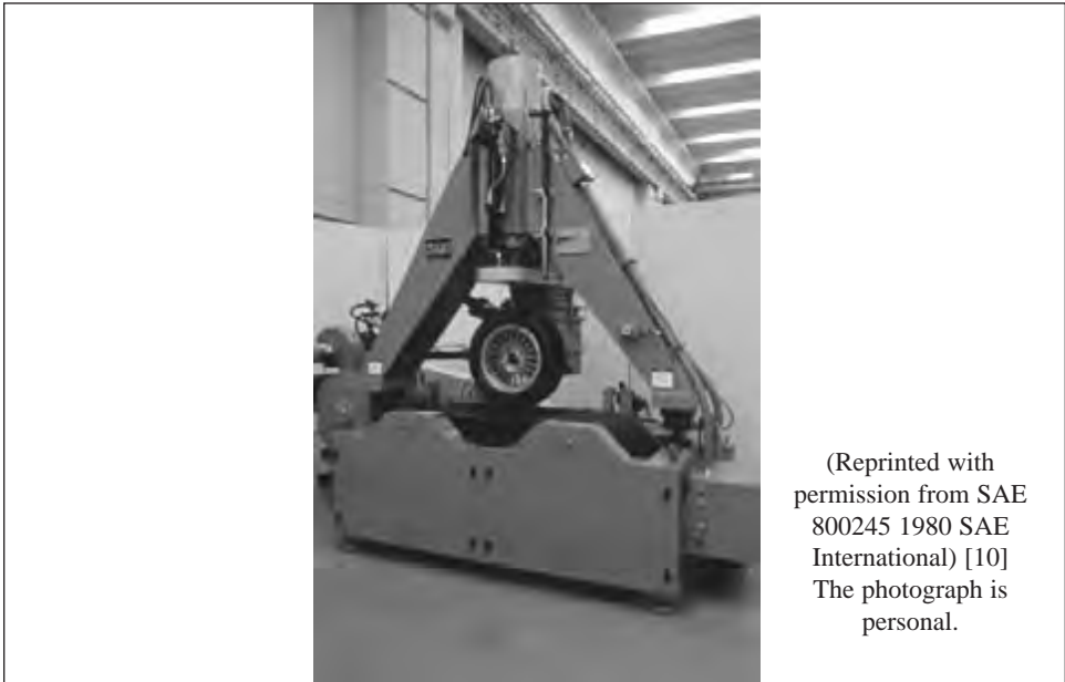
Figure 8.14: The flat-trac I machine, the original Flat-Trac
