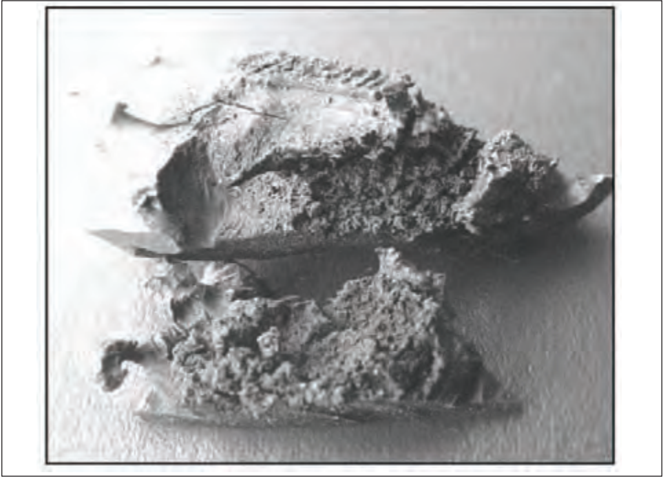
Figure 15.7: Examples of reverted tread rubber
