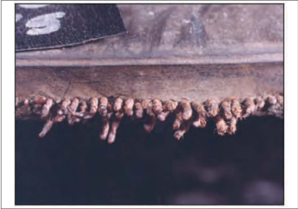
Figure 15.15: Broken, heat-fused polyester body cords, upper sidewall
