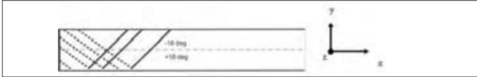
Figure 6.16 - 2 ply [+18, -18] composite specimen
