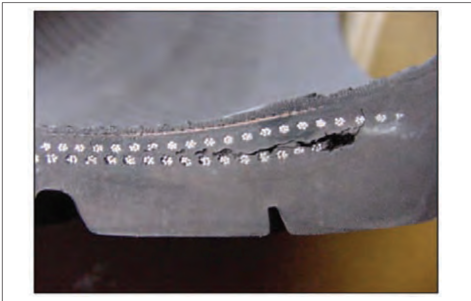
Figure 15.13: Cracking between steel belt edges
