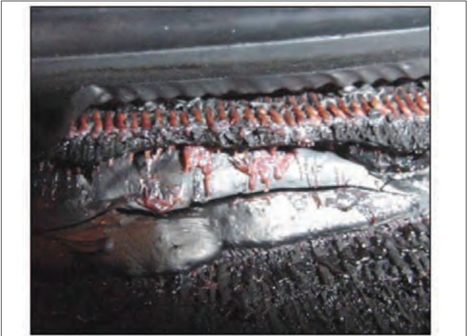
Figure 15.8: Melted polyester cord (lower sidewall)
