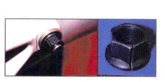
Figure 1: Typical NAS1291 nut application and crack due to hydrogen embrittlement.
