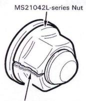
Any crack, if present, would be parallel with nut axis.
