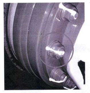
Figure 1 - Example of a failed nut (Courtesy ATSB)
