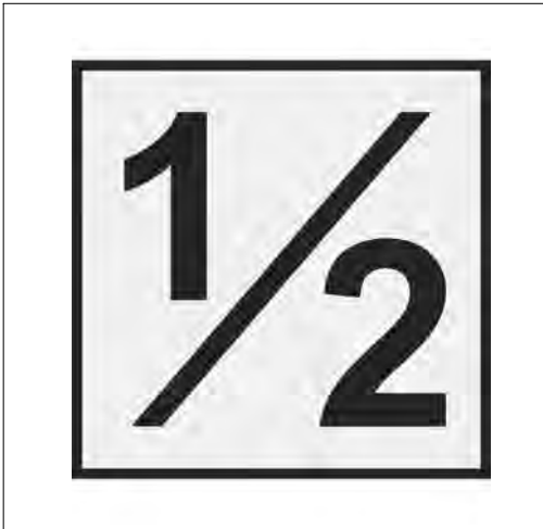
FIG 7-5-1 Typical Runway Half-way Sign
