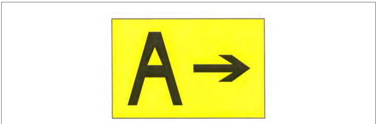
FIG 2-3-36 Direction Sign for Runway Exit
