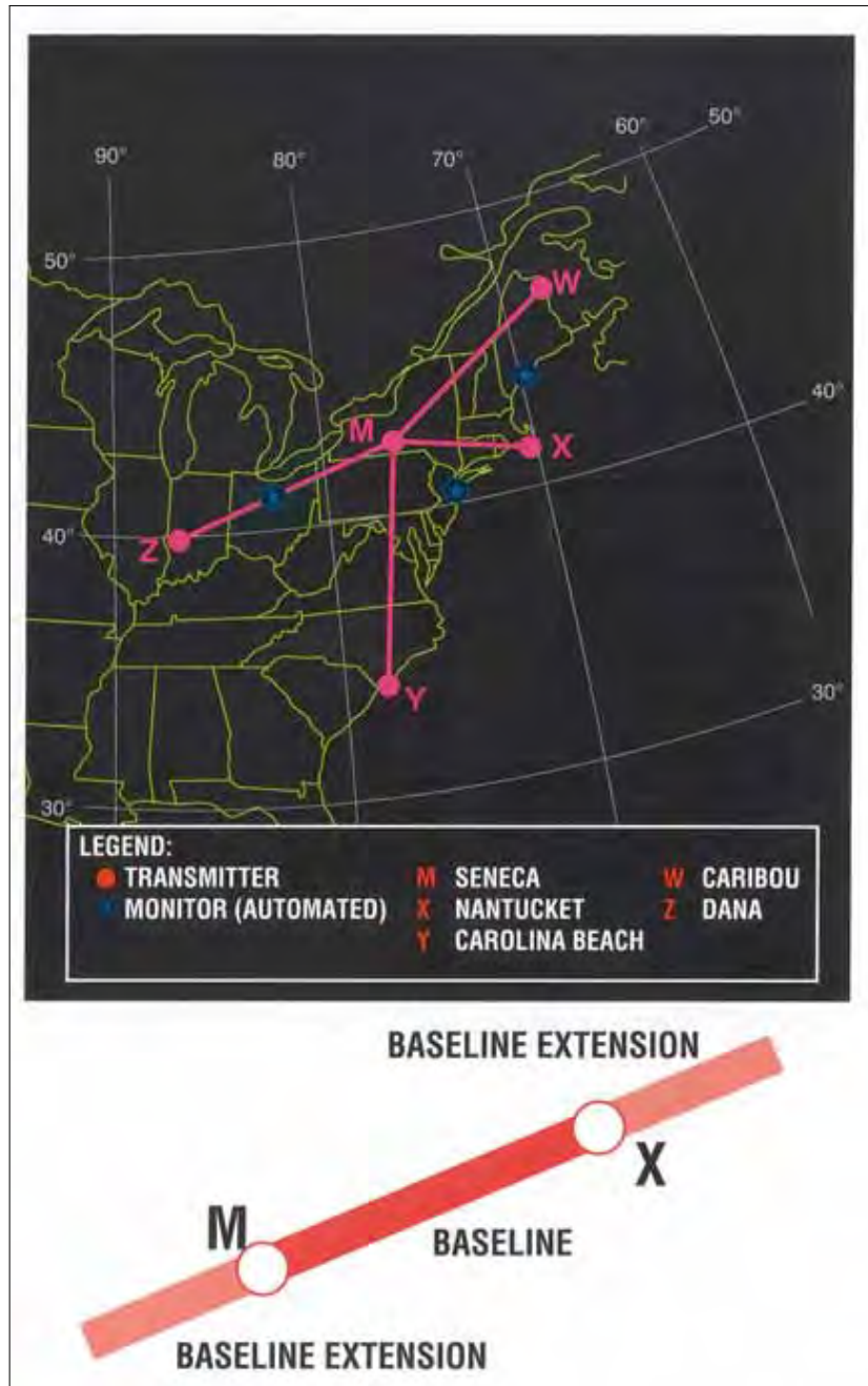
FIG 1-1-14 Northeast U.S. LORAN Chain
