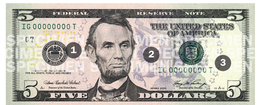
1. Watermark: Column of three smaller numeral 5s 2. Security Thread 3. Watermark: Large numeral 5
