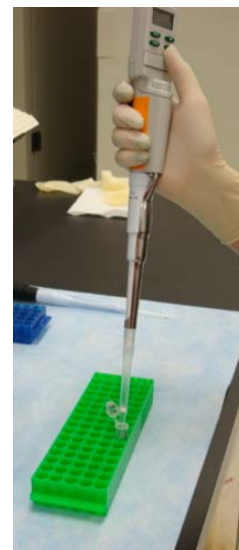
Figure 5: Manual TruTip Method. The TruTip component connected to an electronic pipette for controlled, repeatable fluid flow and ease of use.
