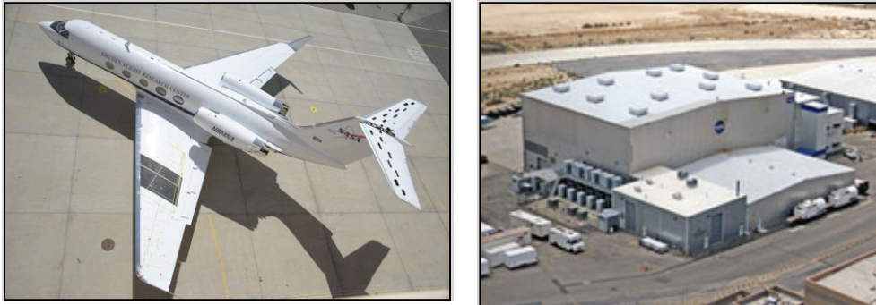
Figure 4. Project testing of airflow (left photo, black section on left wing of the aircraft) at the NASA Flight Loads Laboratory at Dryden (right photo).
