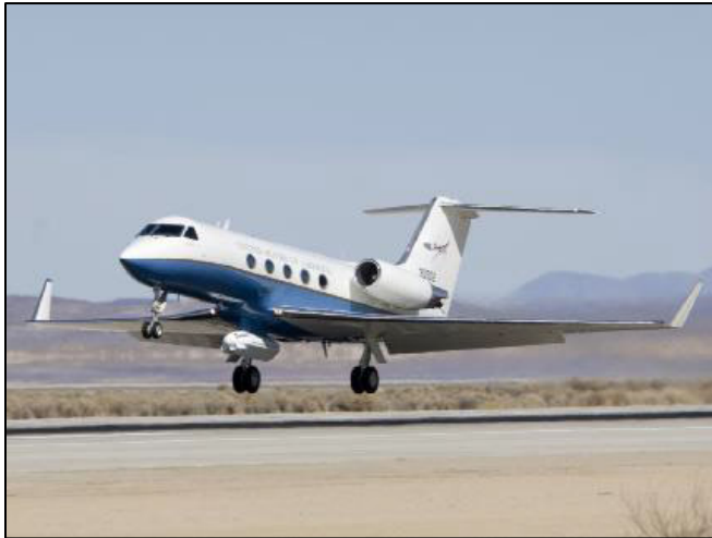
Figure 3. Photo of a NASA Gulfstream III aircraft carrying a synthetic aperture radar pod.
