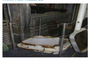
**Open Hatches** are hazardous when not protected. Hatches that are not already protected by coamings at a height of 24 inches, must be guarded (e.g., handrails) at a height of 36 to 42 inches, unless the work being done (e.g., filling fish storage holds) prevents this (29 CFR 1915.73(c)).
