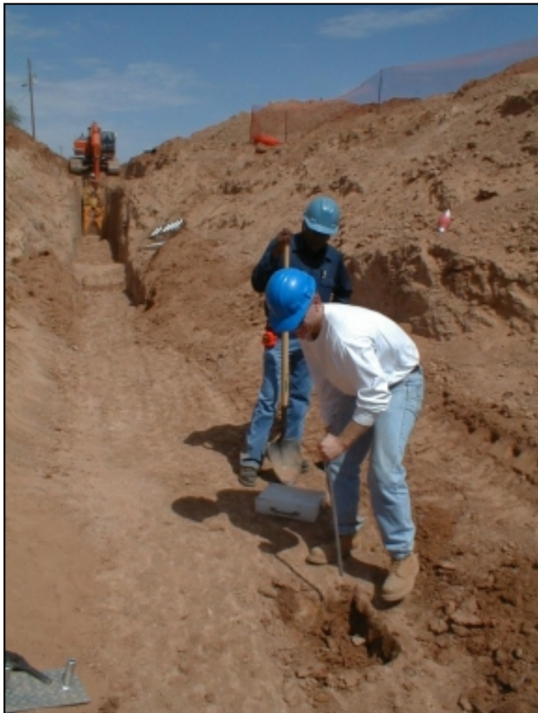
Figure 7: Nuclear density testing on a construction site on the Tohono O'odam Reservation, Arizona.
