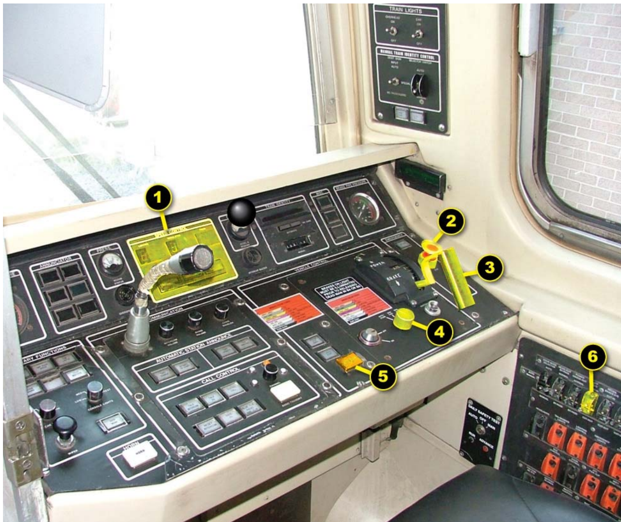
Figure 3. Exemplar Rohr 1000-series car operator's console: (1) speed control indicator panel, (2) emergency brake "mushroom," (3) master control handle, (4) mode director switch, (5) automatic train operation stop, and (6) automatic train protection cutout switch.
