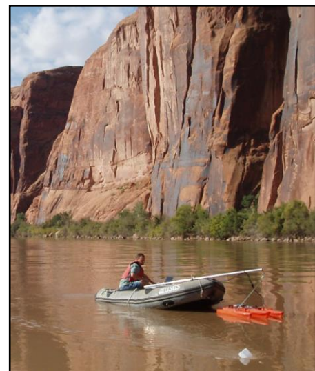
Figure 8 – Acoustic Doppler Current Profiler discharge measurement on the Colorado River above Kane Creek
