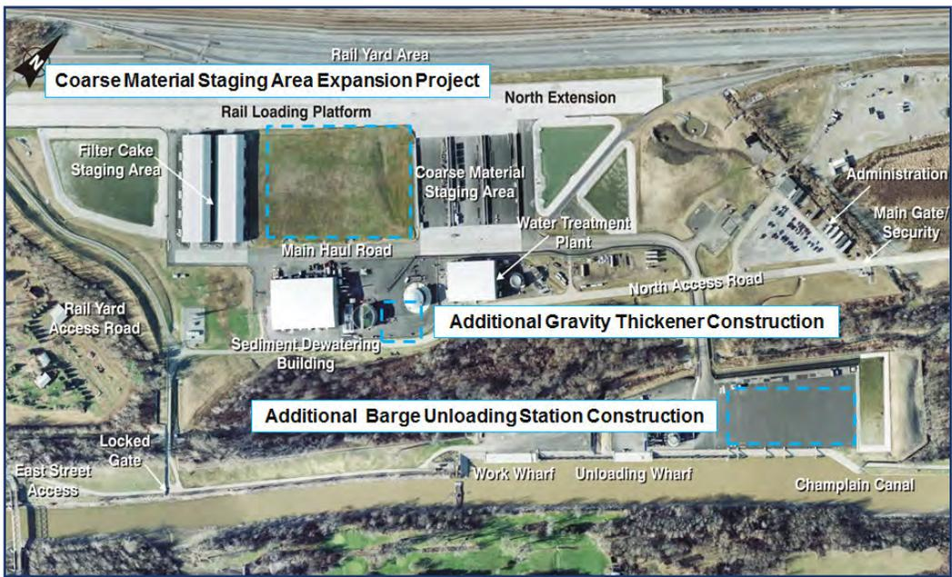
**Figure 2:** Processing Facility improvements for winter/spring 2012 include expansion of the coarse material staging area and construction of a second barge unloading station, additional size separation equipment, and a second gravity thickener.
