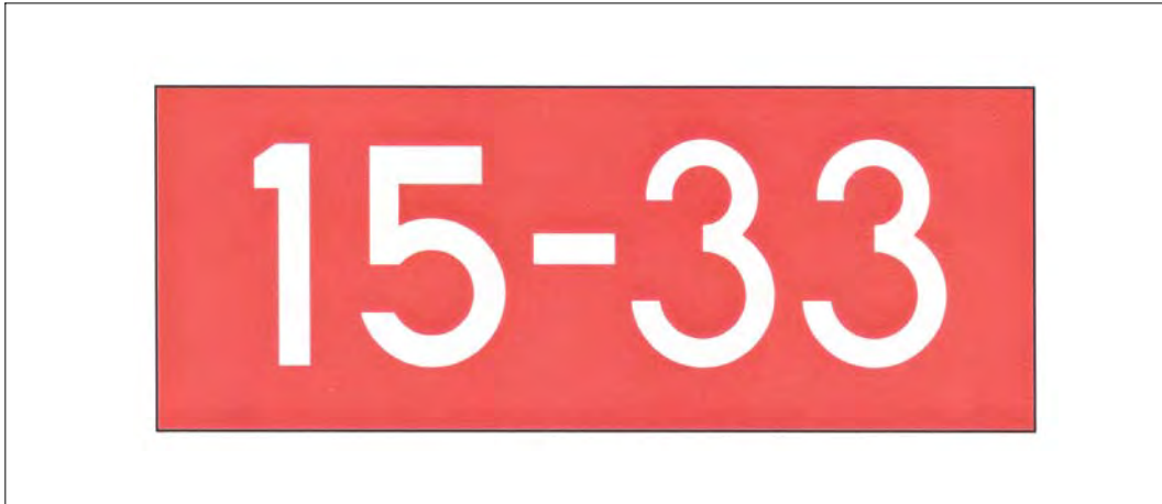
FIG 2-3-24 Runway Holding Position Sign
