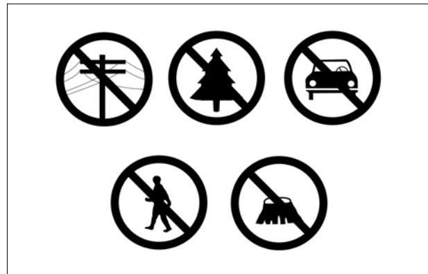
Landing Zone Hazards
