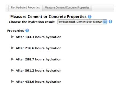
When one of these individual sections is expanded, it reveals two buttons, one to calculate the elastic properties (effective linear elastic moduli) and one to calculate the transport properties (effective diffusivity). Clicking on these buttons launches the finite element models that calculate these properties on the digital image [Garboczi 1998].
