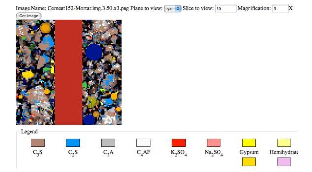
**Plane to view**: Choose one of three orthogonal directions from which to view the microstructure. The viewing planes are defined by the two Cartesian coordinate axes they contain (e.g., the yz plane is the plane observed when viewing along the x-axis).
