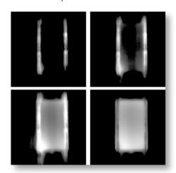
machining conditions. To this end, the Metallurgy Division has worked with the Manufacturing Engineering Laboratory to develop measurement methods for the deformation behavior of steels at high strain rate during extremely high heating rates using a unique, electrically pulse-heated Kolsky bar.
