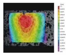
DIC Measurement of Tissue Simulant Material
