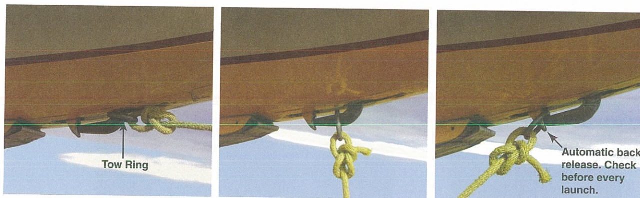
Figure 7-13. Testing the towhook.
