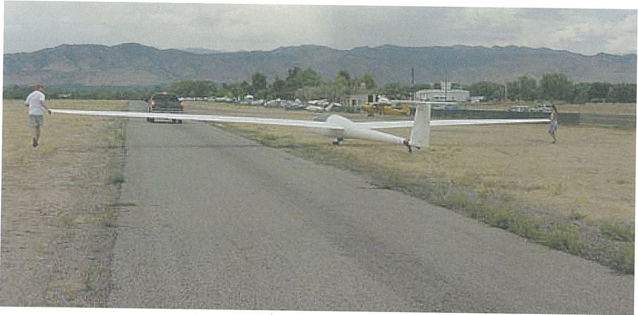
Figure 6-5. Positioning the glider for the tow vehicle.
