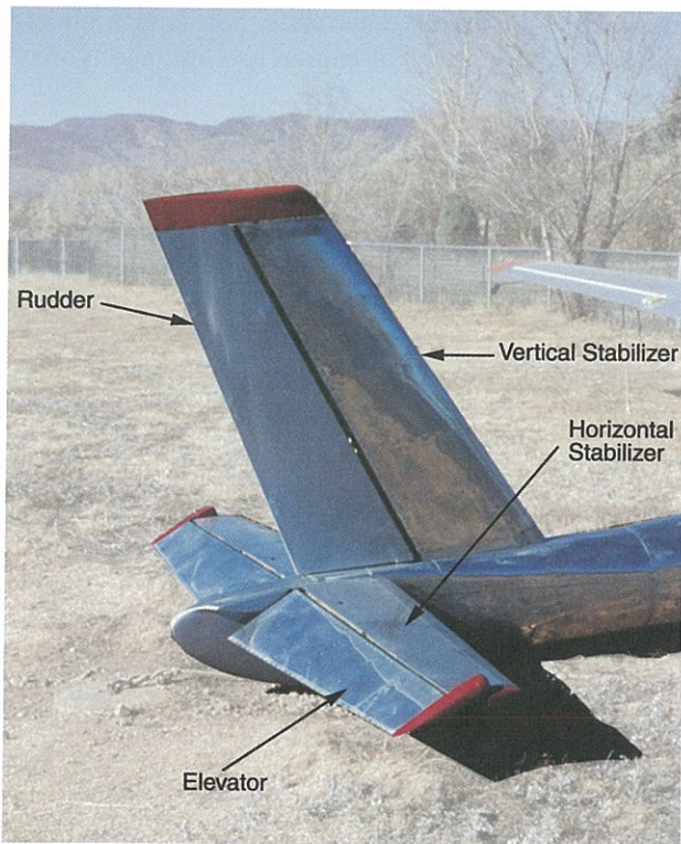
Figure 2-4. The empennage components.
