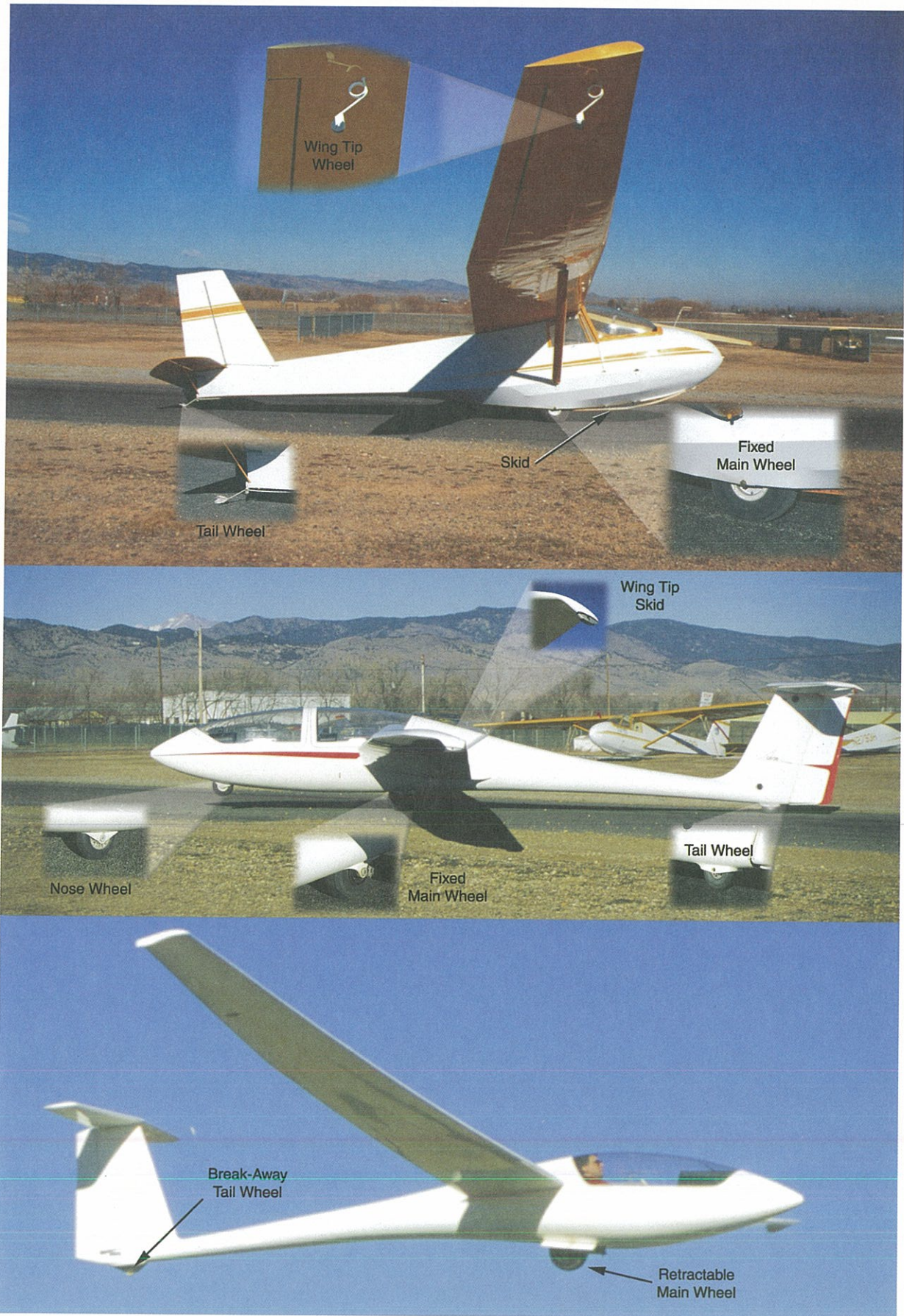
Figure 2-8. Some gliders have fixed main wheels, others have retractable main wheels. Nose skids, or nose wheels, tail wheels and wing tip wheels are found on many gliders.
