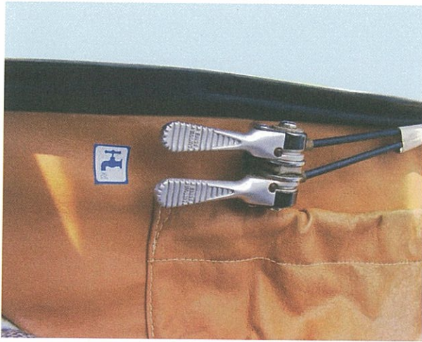
Figure 5-20. Water ballast drain valve handles.
