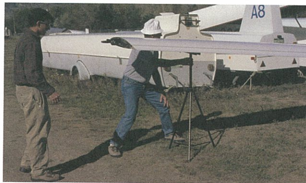
Figure 6-1. Wing stand used during glider assembly.
