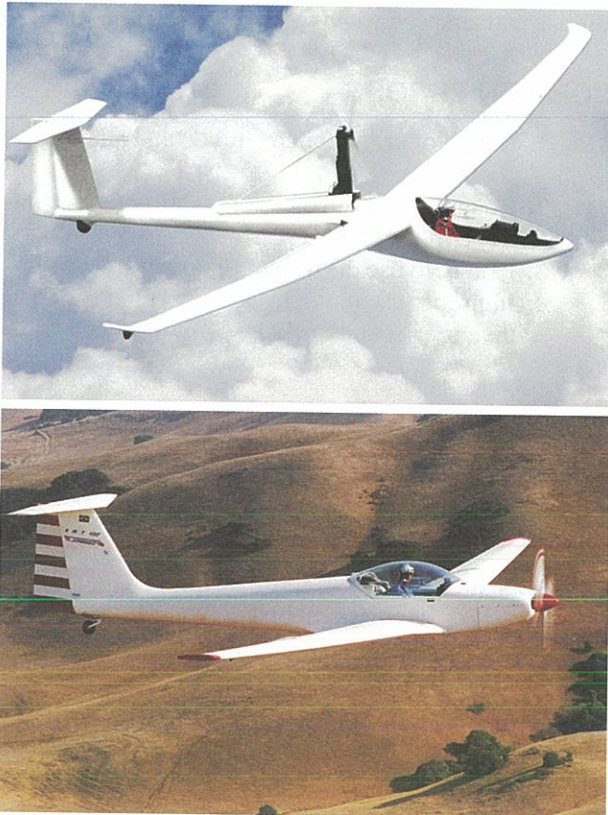
Figure 7-24. Types of self-launch gliders.
