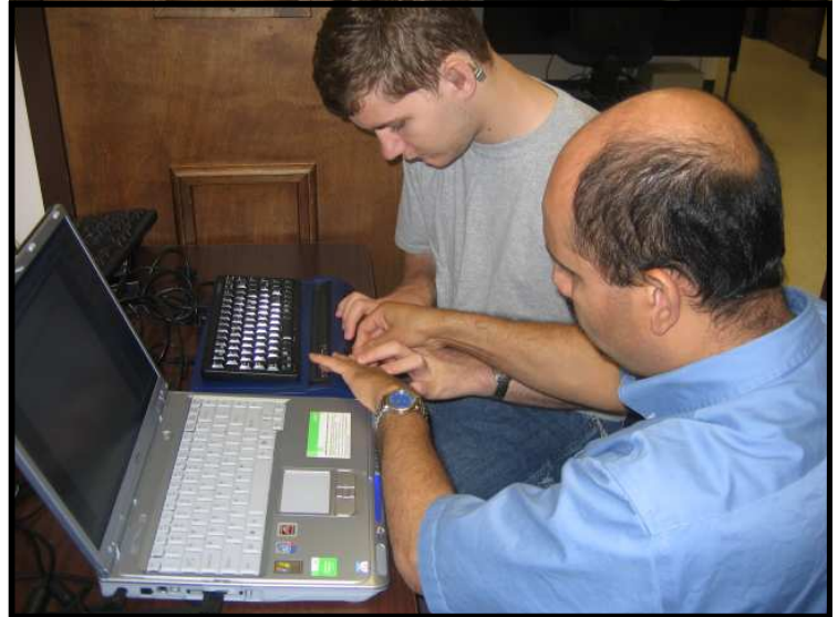
A technology instructor helps his student find the braille cells on his refreshable braille display.
