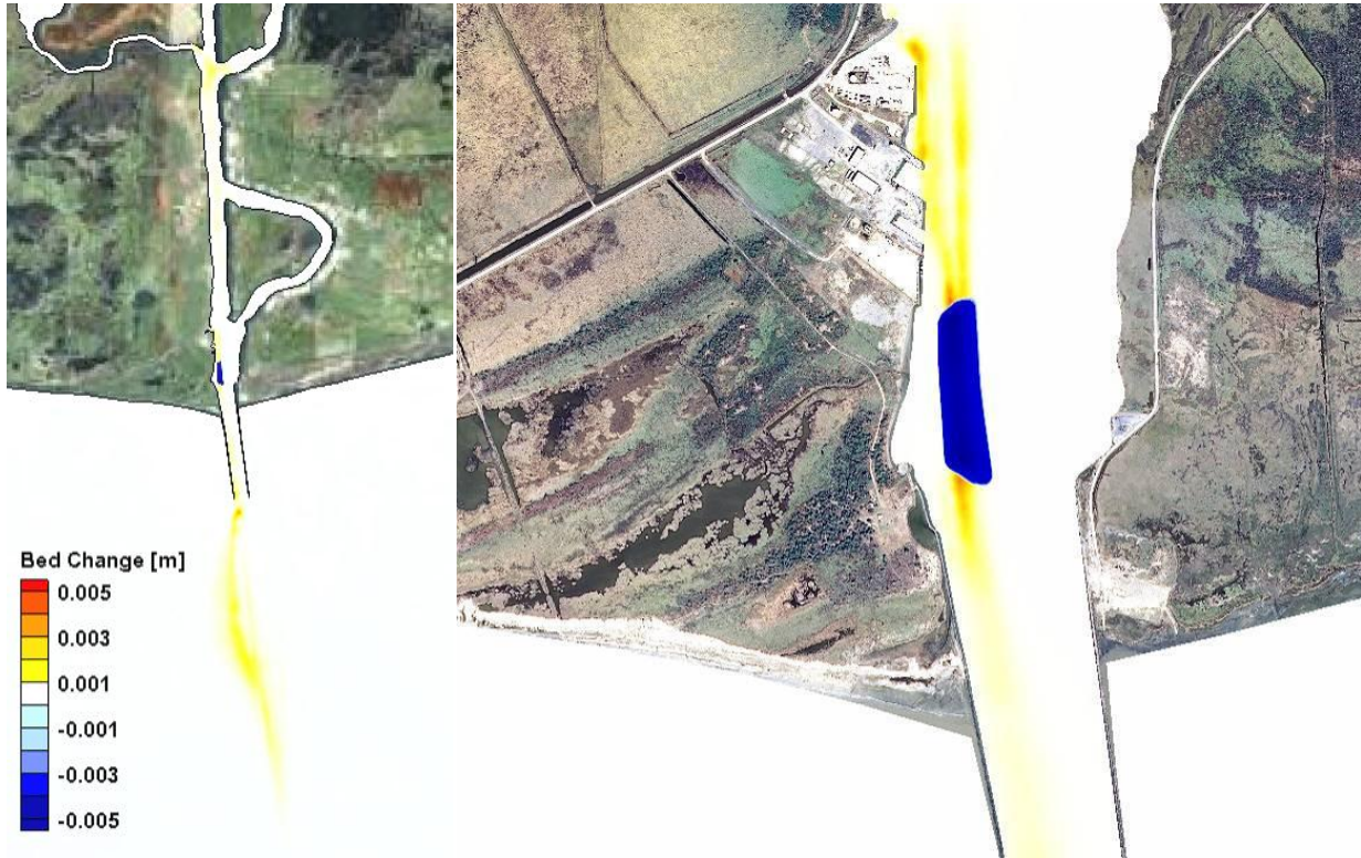
FIGURE 8 BED CHANGE RESULTING FROM FIVE MONTHS OF SEDIMENT TRANSPORT FROM THE RE-HANDLING SITE
