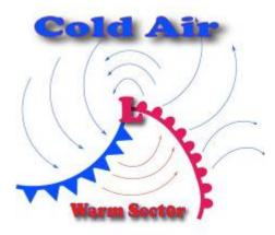
The illustration shows the "classic" northern hemisphere low pressure system with the associated cold and warm fronts. Remembering that air circulates counterclockwise around a low pressure system in the Northern Hemisphere will help you visualize the overall temperature, wind, and moisture patterns in a given area. Because weather is associated with fronts, which are in turn associated with low pressure systems, you can get some idea of possible conditions just by looking to see where the low
