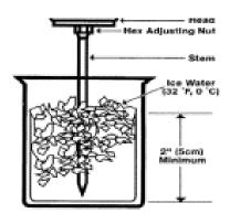
removing the stem from the ice, hold the adjusting nut under the head of the thermometer with a suitable tool and turn the head so the pointer reads 32 °F.
