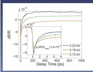
Degenerate pump-probe-reflectivity measurements at 3 different photon energies at room temperature. The inset displays the early time dynamics, with two identical vertical bars that represent the maximum difference between the signals at the highest and lowest pump photon energies. The signals reach their maximum difference at 3 ps.
