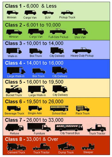
FIGURE 58. Examples of Trucks in Each Truck Class
