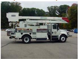
FIGURE 81. Hybrid Bucket Truck
