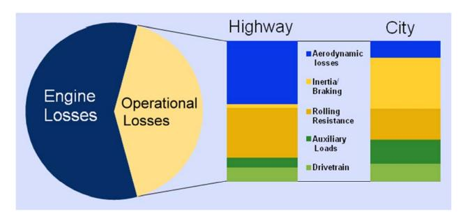
FIGURE 84. Class 8 Truck-Tractor Energy Losses
