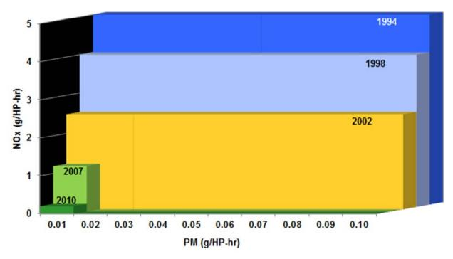
FIGURE 106. Diesel Emission Standards, 1994-2010
