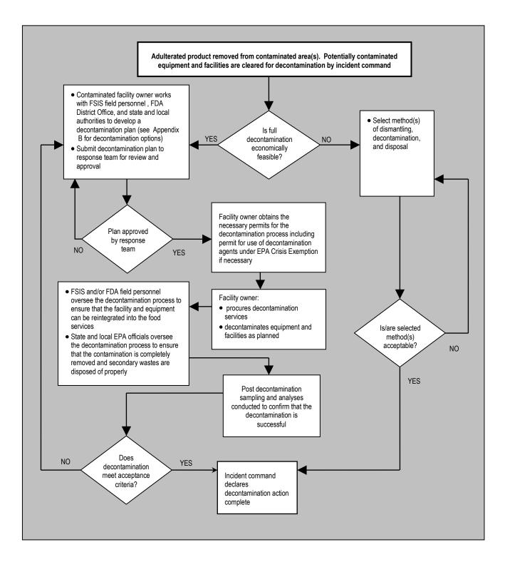
Figure 4–3. Decontamination Phase
