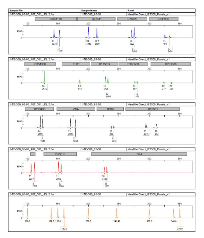
Only one sample produced a full DNA profile, but due to the data being off scale, artifacts (pullup) were also present. Quantitation results for the remaining three samples were very low, which explains why they did not provide a full DNA profile.
