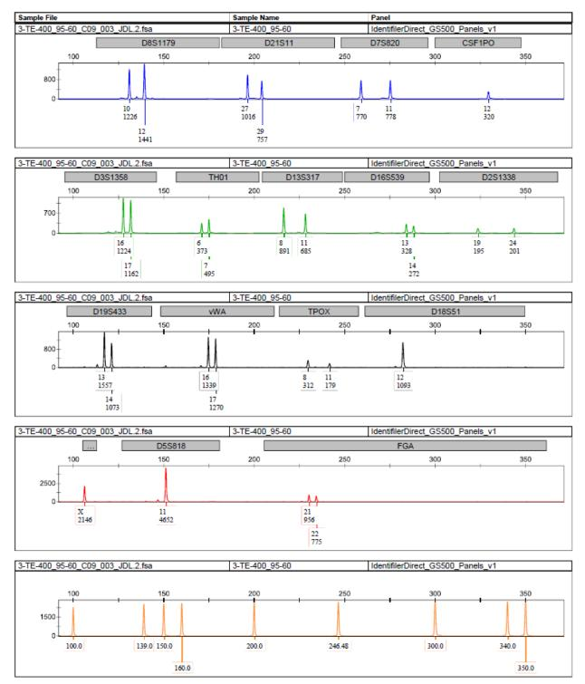
In methods 3 and 4, it was expected that the DTT present was inhibiting the amplification. The SEB concentration used is 2% which should be tolerable according to Applied Biosystems<sup>™</sup>. To verify this theory, method 19 used a lysing reagent of SEB with no DTT. None of the samples had peaks present, indicating a complete amplification failure. This proves the SEB is causing inhibition in the amplification.
