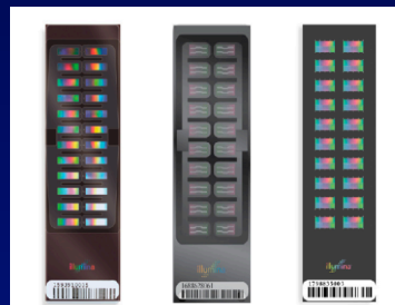
Infinium Assay BeadChips enable interrogation of >317,000 to over one million SNPs and offer comprehensive coverage of CNV regions. Shown above, from left to right, are the Human1M, Human150-Duo, and Human550-Duo BeadChips.
