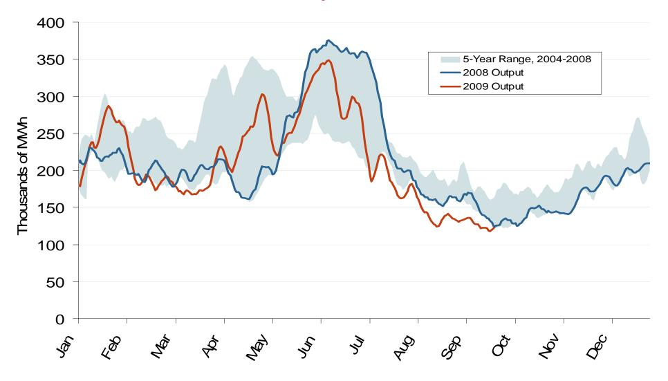
Source: Derived from *USACE* data reflecting the output of the 24 largest facilities. Trend lines are 7-day moving averages.
