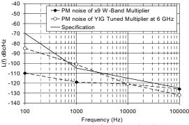
**Figure 6:** PM noise of ×9 W-band GaAs multiplier at 90 GHz and YIG tuned multiplier at 6 GHz. The noise of these components adds directly to the Gunn oscillator noise.
