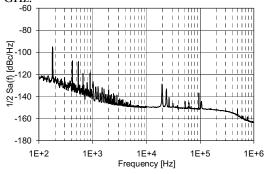
**Figure 8:** AM noise of locked Gunn oscillator at 94 GHz.
