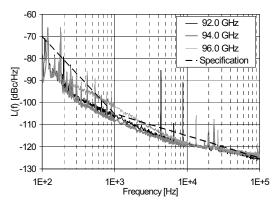
**Figure 5:** PM noise of locked Gunn oscillator at different frequencies. Measured phase noise is combined noise of a pair of similar oscillators. Noise of single oscillator is 0 to 3 dB better than shown.
