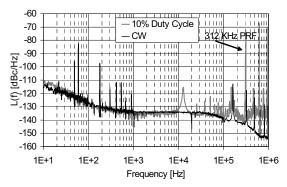
**Figure 9:** PM noise of InP Amplifier at 94 GHz, Pin = -2.5 dBm and PRF = 312 kHz.
