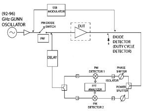
**Figure 1:** The residual PM noise of an amplifier (DUT) is measured with the configuration shown. Mixer and isolator noise in the top PM detectors are uncorrelated with respect to the bottom detectors. The PM noise of the (92-96) GHz oscillator signal is suppressed, since it appears equally at both inputs to the mixers.
