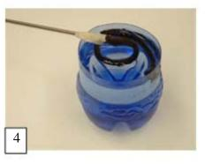
2. Assemble the wet bulb thermometer. Cut a portion of the wicking material (it should be long enough to reach the bottom of the water vessel and than some). Connect the sensing portion of your temperature recorder to the wick by inserting the probe/wire/stem into the center of the wick (image 2). Secure the end of the wick to the probe/wire/stem using tape. Place the wick in the water-containing vessel. Make sure the wick is completely
