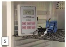
reading temperature measuring device to make process adjustments, place the wet bulb thermometer for easy access and readability, such as near a door or window (image 5). If immediate feedback is not a consideration (image 6), place the device where the ambient conditions of your process are least likely to give you optimum conditions - hence a "worst case" reading. Position the wet bulb thermometer in a flow of air (such as
