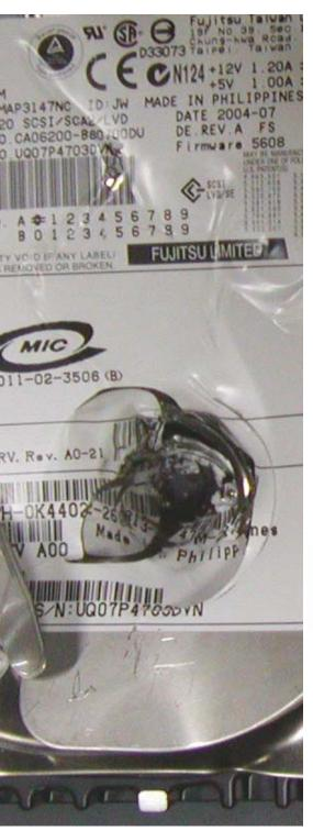
The FRCs' hydraulically-loaded crushing machines can completely physically destroy your agency's hard drives. The crusher uses 12,000 pounds of force to produce a conical punch that causes catastrophic trauma to the hard drive chassis while also destroying the internal platter. This force is sufficient to mutilate the drive so that it cannot be reconnected or reinserted into a functioning computer.
