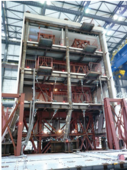
Figure A-15 Collapse due to dynamic instability (courtesy of D. Lignos).
