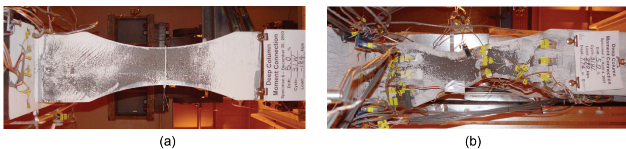
Figure A-4 Results from connection tests of RBS beams with deep columns: (a) balanced panel zone design; (b) strong panel zone design (Ricles et al., 2004a).
