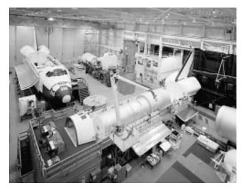
High angle view of Building 9 Training Facilities including the Space Shuttle Full Fuselage Trainer and the Remote Manipulator System (RMS) mock-up. Also visible is a mock-up of the Hubble Space Telescope for use in training with the RMS.
