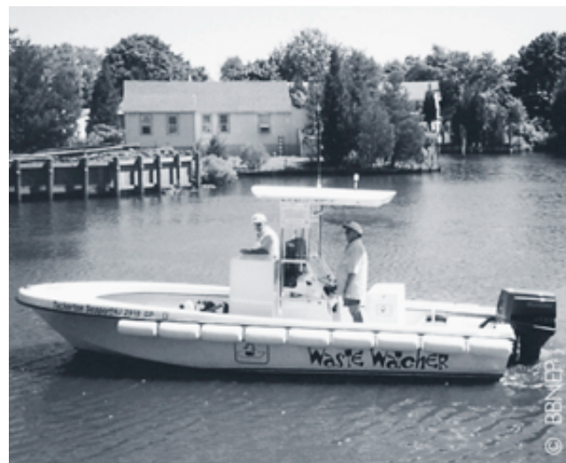
Mobile pump-out stations, such as the boat shown here, help reduce sewage discharges to Barnegat Bay (BBNEP).
