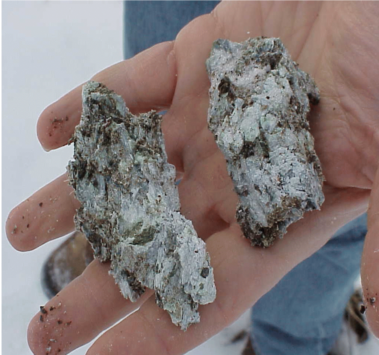
Figure 2. Photograph of a sample of Libby, Montana, vermiculite ore. Fiber-like structures can be seen along the left edge of the piece of ore on the left. Source: U.S. Geological Survey and U.S. Environmental Protection Agency, Region 8, Denver, Colorado.
