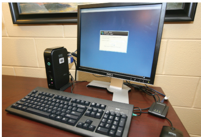
Student living quarters will contain computer systems called Thin Clients. These systems are centrally controlled by a unique server that stores information for multiple computers.
