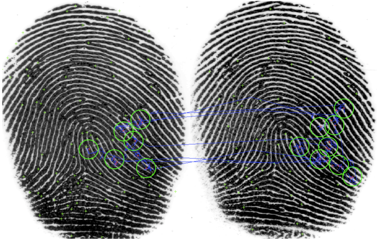
Figure 12. Graphical illustration of counting nearby minutiae. The Universal Latent Workstation was used to computer-code the locations of the minutiae, shown here as green crosses. We then determined the fixations for each user (shown as red crosses) and counted the number of minutiae contained in a circle centered on each fixation (green circles).
