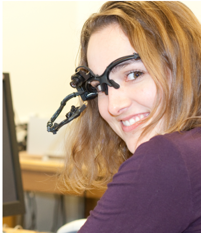
Figure 2. Our eye tracker worn by a participant in the eyetracking studies. It consists of one camera that monitors the position of the eye relative to the head, and a second camera that monitors the position of the head relative to the images being examined.
