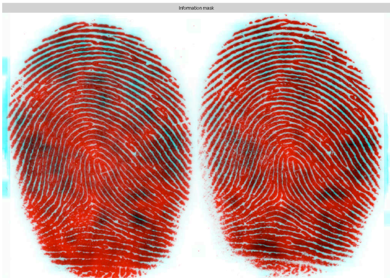
Figure 21. The information contained in the absolute orientation of ridge elements. Red regions are those that are more informative by this measure.
