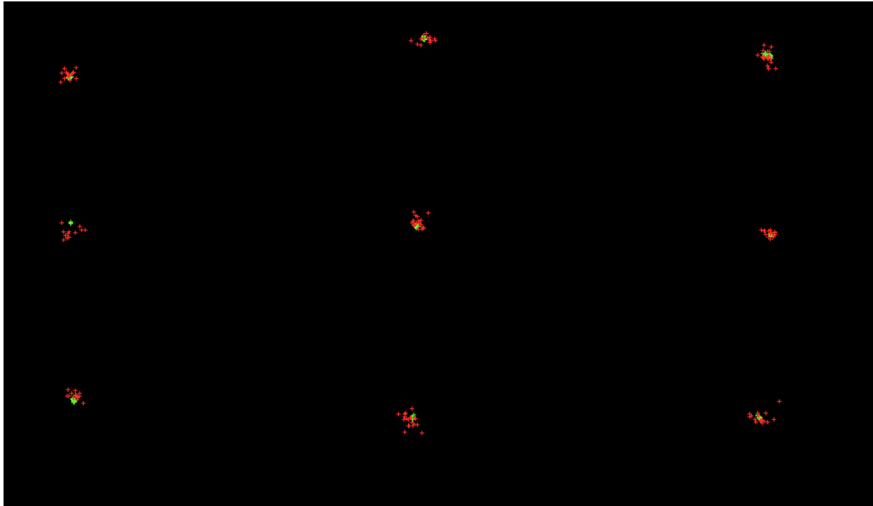
Figure 9. Results of the calibration procedures. Green dots are locations on the monitor that were fixated, and red dots are the estimated eye positions. The close clustering of each set of red dots illustrates the accuracy of our system, which is comparable to commercial systems. We typically see error on the projected monitor of less than 1 degree of visual angle and often less than .5 degrees, which is similar to commercial systems such as the Tobii system.
