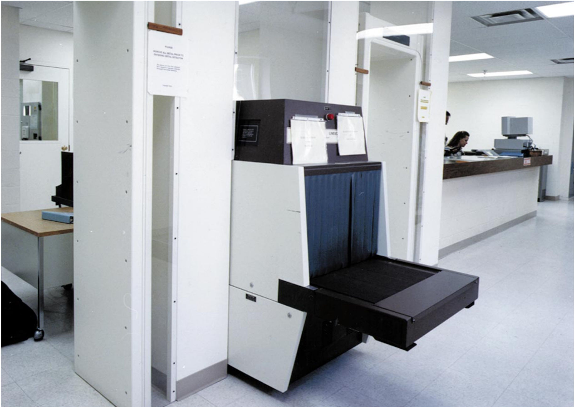
Exhibit 2.18. A weapon detection system with x-ray detector for carried items and two portal metal detectors for walk-through.
