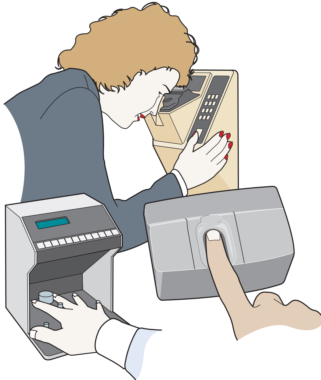
Exhibit 4.4. Illustrated here are several types of biometric identifiers that can be used for entry control with a high confidence of accuracy.
