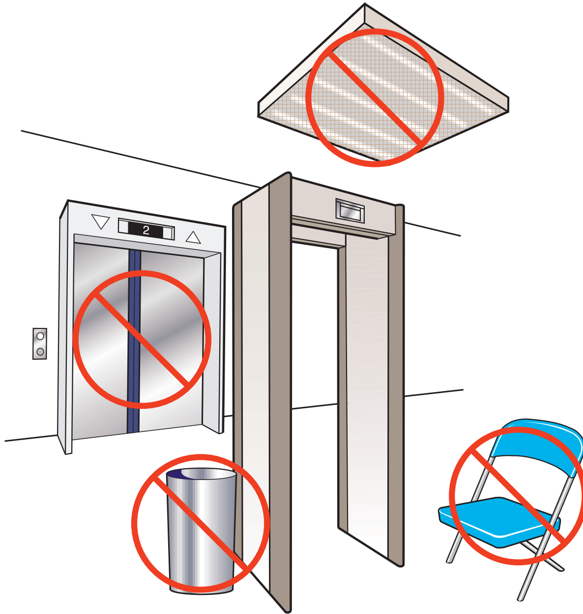
Exhibit 3.8. Portal metal detectors are subject to many sources of interference that can reduce their sensitivity if not compensated for in the initial programming.
