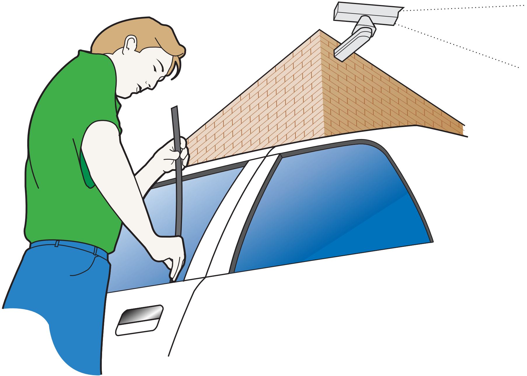
Exhibit 2.6. A pan-tilt-zoom camera that is set to automatically pan an area may completely miss capturing incidents of concern.
